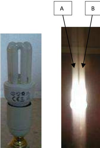
Figure 6: lamp 11W 600Lm 80mA 220-240V ~ 50/60Hz (left) two beams of light A and B (right)
