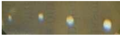
Figure 15: sunlight move through pattern reflects spot images on hexagonal crystal. Crystal placed 1 cm behind pattern.
