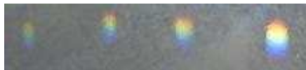
Figure 18: sunlight move through pattern reflects spot images on hexagonal crystal. Crystal placed 4 cm behind pattern.
