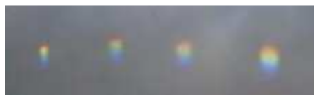
Figure 21: sunlight move through pattern reflects spot images on hexagonal crystal. Crystal placed 7 cm behind pattern.
