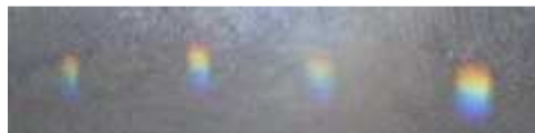
Figure 20: sunlight move through pattern reflects spot images on hexagonal crystal. Crystal placed 6 cm behind pattern.
