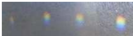
Figure 19: sunlight move through pattern reflects spot images on hexagonal crystal. Crystal placed 5 cm behind pattern.
