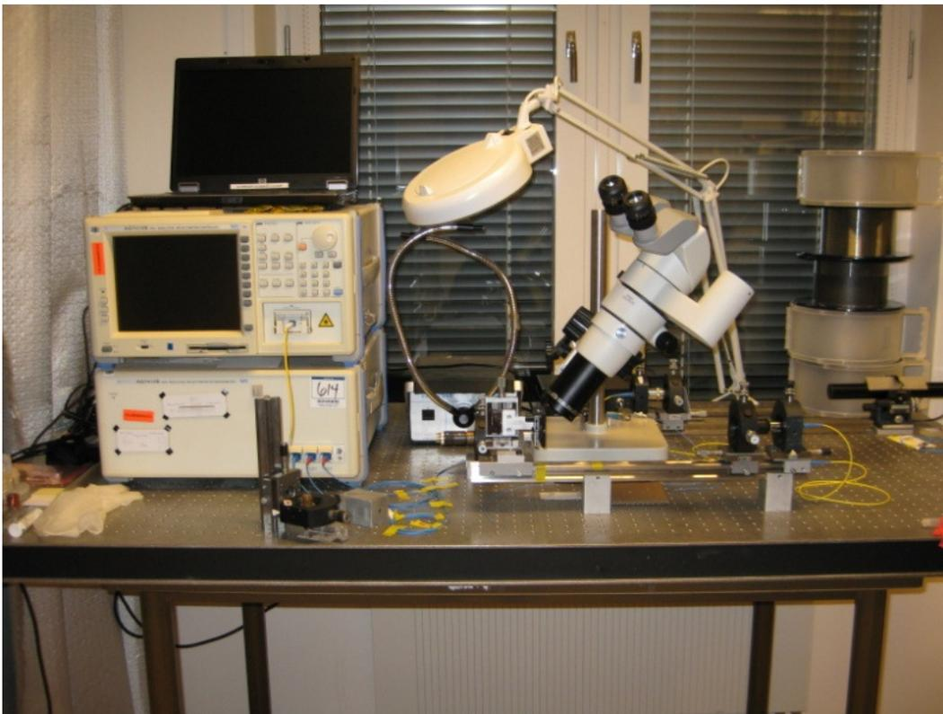
*Figure 10: An image of the Ando AQ7410B Reflectometer*
